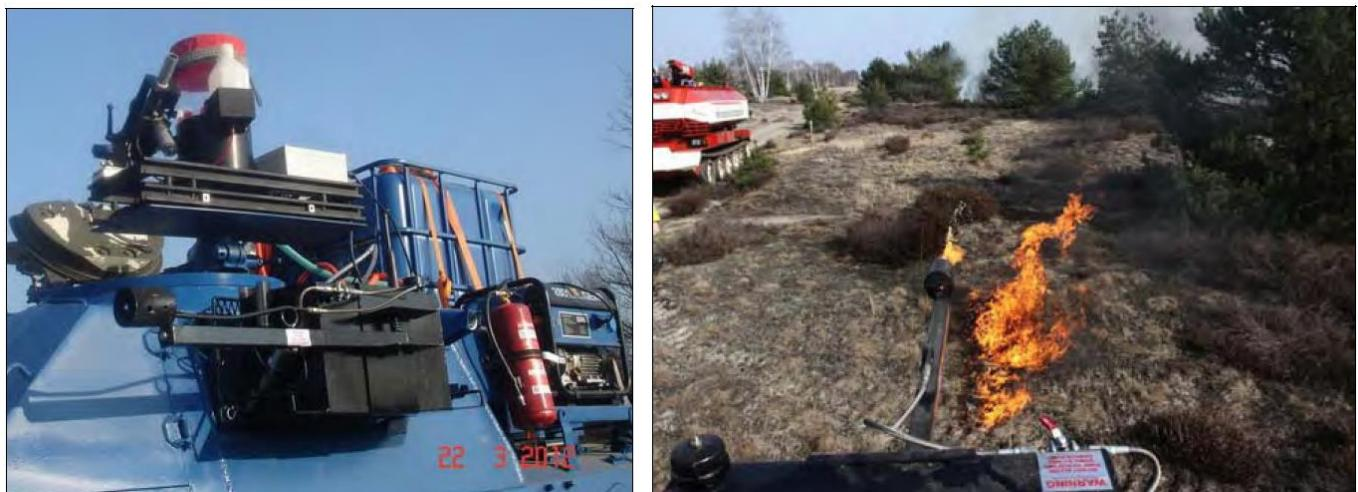
**Figures 2.24 to 2.25.** Converted BMP-OT-R5 tank for use as armored ignition tank, equipped additionally with an ATV drip torch to set prescribed or back fires. Photos: GFMC.
