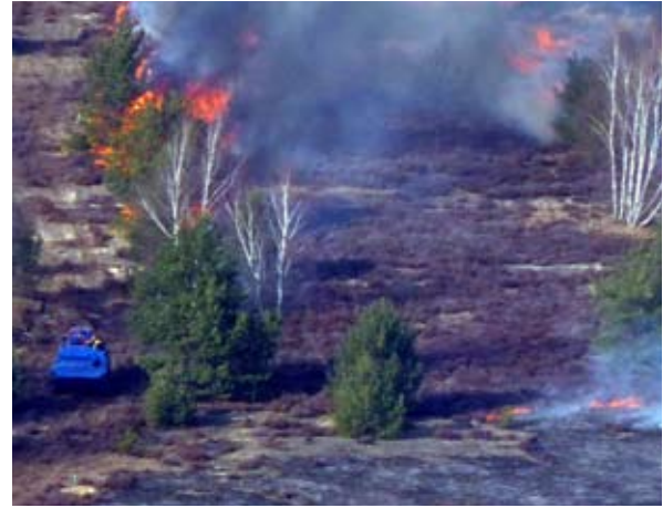
Figures 34 and 35 – UAV-supported ground operations: The manned, armored ignition tank (blue) and the fire suppression tank (red-white) are directed via drone control. GFMC operations in Brandenburg State, Germany, on former military shooting ranges and WW-II combat theatres. Photos: GFMC.
