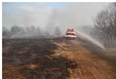
Figures 37 to 39 – Use of the SPOT-55 firefighting tank, a converted T-55 with 11,000 l of fire suppressant (water, foam) operated by DiBuKa, Germany, to safely control prescribed fires or wildfires on UXO- and radioactivity-contaminated terrain. Photos: GFMC.
