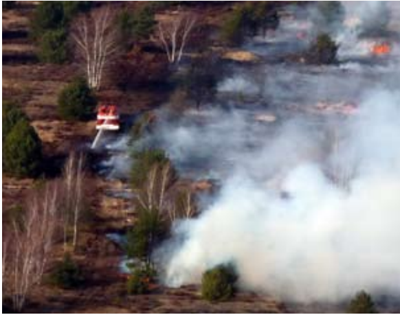
Figures 34 and 35 – UAV-supported ground operations: The manned, armored ignition tank (blue) and the fire suppression tank (red-white) are directed via drone control. GFMC operations in Brandenburg State, Germany, on former military shooting ranges and WW-II combat theatres. Photos: GFMC.
