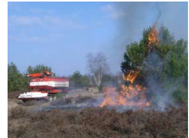
Figures 37 to 39 – Use of the SPOT-55 firefighting tank, a converted T-55 with 11,000 l of fire suppressant (water, foam) operated by DiBuKa, Germany, to safely control prescribed fires or wildfires on UXO- and radioactivity-contaminated terrain. Photos: GFMC.
