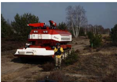
Figures 37 to 39 – Use of the SPOT-55 firefighting tank, a converted T-55 with 11,000 l of fire suppressant (water, foam) operated by DiBuKa, Germany, to safely control prescribed fires or wildfires on UXO- and radioactivity-contaminated terrain. Photos: GFMC.
