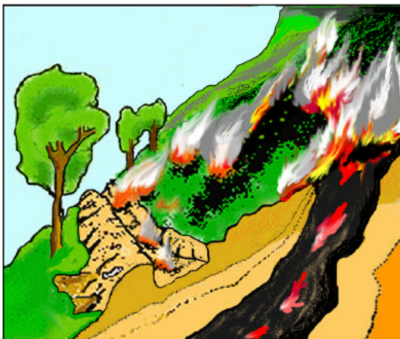
Figure 5. Undercut fire trench built below the line of a burning coal-seam that runs horizontally across a slope.
