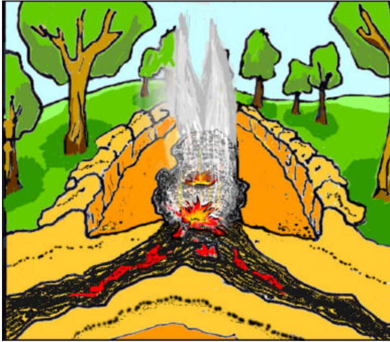
Figure 4. Undercut fire trench dug down to mineral soil to isolate a coal-seam fire.
