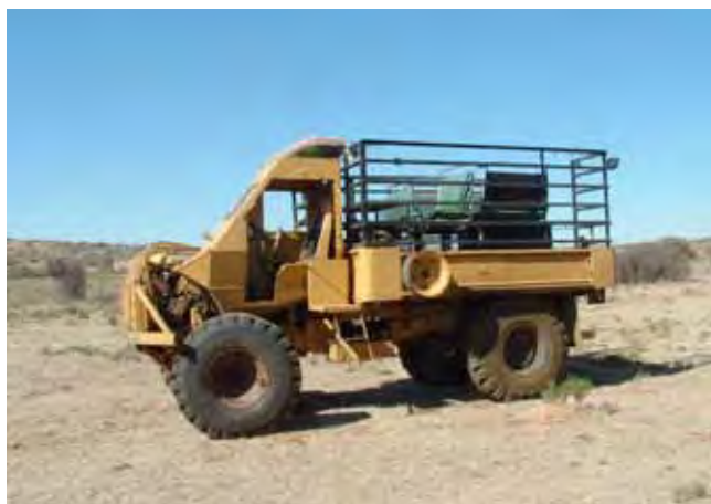
Figure 7.2. A locally-manufactured fire truck operating in a farming region, structured on the chassis of an old Defense Force truck. Photo: C. de Ronde.
