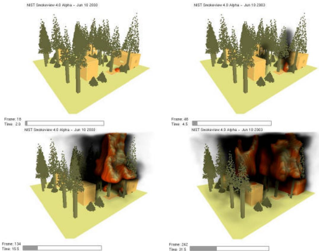
Figure 4 Selected frames from FDS / Smokeview simulation of “neighbourhood scale” fire spread from a single ignition. The fire spreads from ground fuels, through ladder fuels to the tree-crowns. Structures are ignited by heat flux from the burning vegetation.
