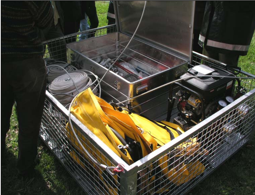
Figure 5. Forest fire tool box for the use at higher elevations with bad access or too long-lasting driving distances - to be transported with helicopter support.
