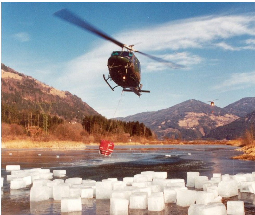
Figure 6. Heli-supported fire suppression during the Stagor mountain fire (on a former stand-replacing storm event near Steinfeld, February 2002). The photograph shows water filling operation at the Weissensee in Southern Carinthia. Access to water was possible only after part of the thick ice layer was sawn and the many resulting ice blocs put on the lake ice (in the foreground).
