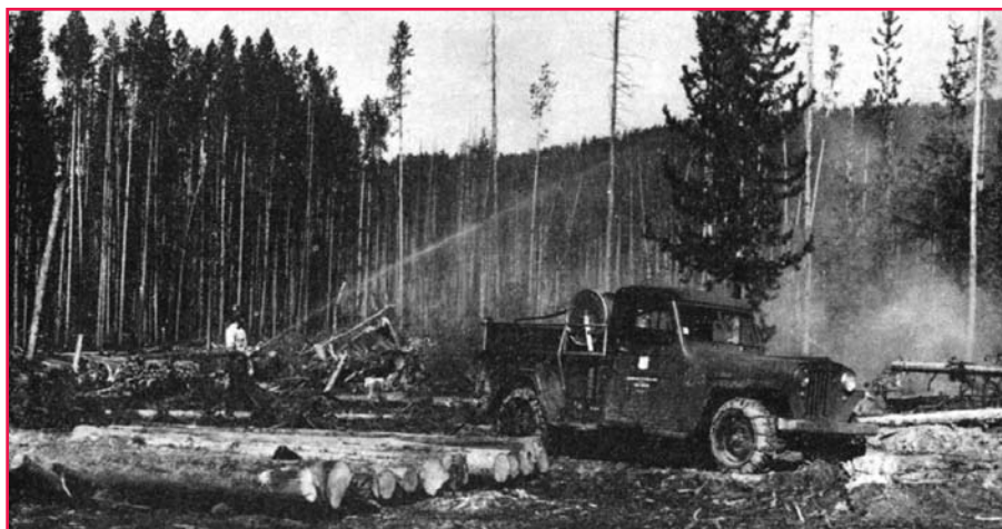
Figure 2 —A jeep tanker being tested prior to the broadcast burning of an area of lodgepole pine slash on the Deerlodge National Forest in Montana. Photo: USDA Forest Service.
