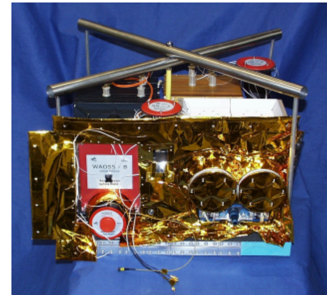
Payload platform of the flight model with assembling tools Total mass: 30.2 kg
