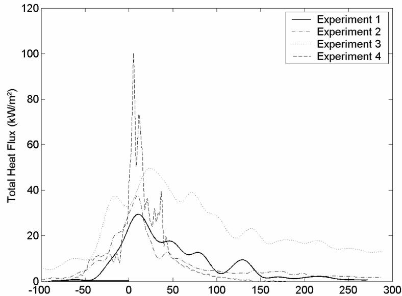
**Figure 4**—Flux-time measurement for the four fire spread experiments
