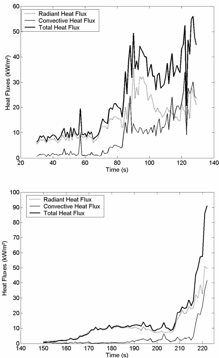
**Figure 5**—Flux Comparison of the radiative and convective heat fluxes as fire approaches for experiment 3 and 4
