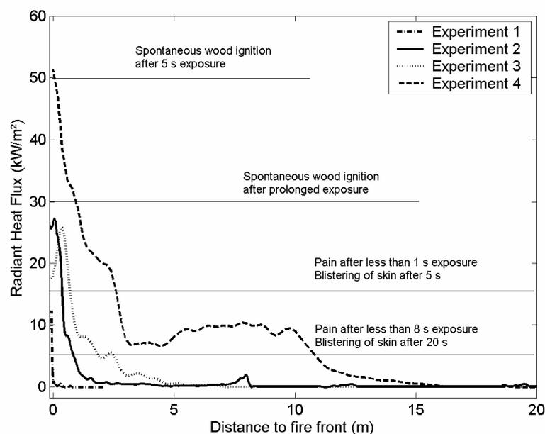
Figure 6—Distribution of the incident radiation ahead of the fire front
