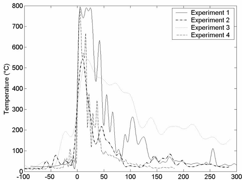
**Figure 3**—Temperature-time measurement for the four fire spread experiments
