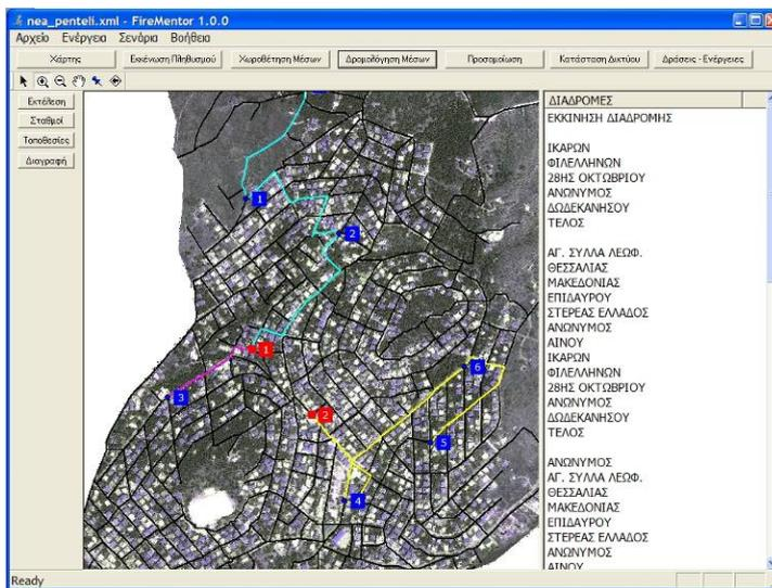
Figure 8. Service unit routing
