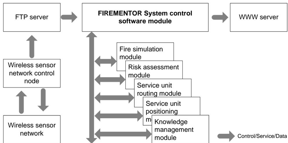
Figure 9. *Firementor* software modules architecture
