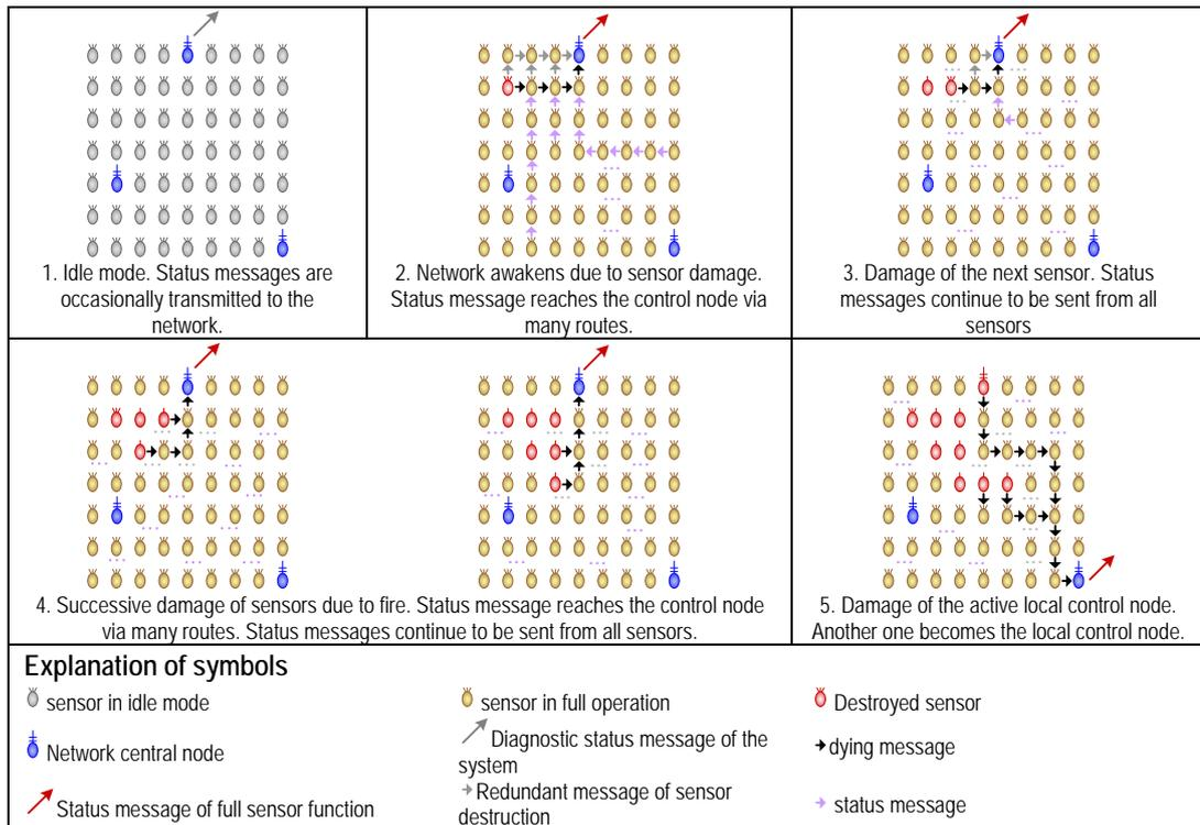
**Figure 3.** Message routing in the *Firementor* in-situ measurement network
