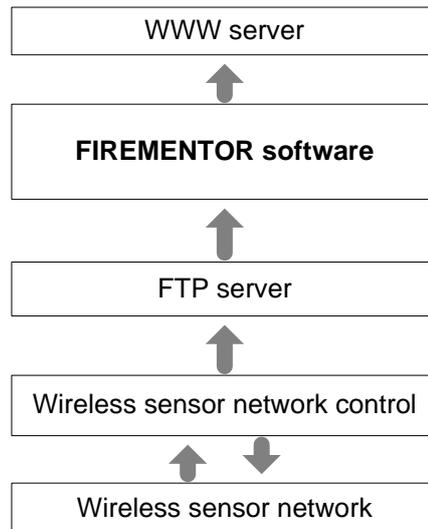
Figure 1. Block structure of the *Firementor* system
