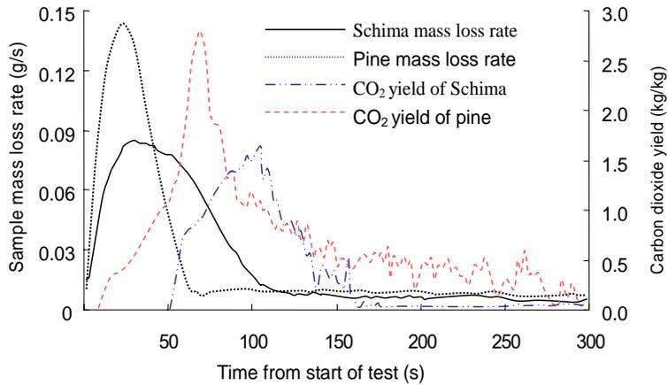
Figure 5 Mass loss rate and carbon dioxide yield of the two samples
